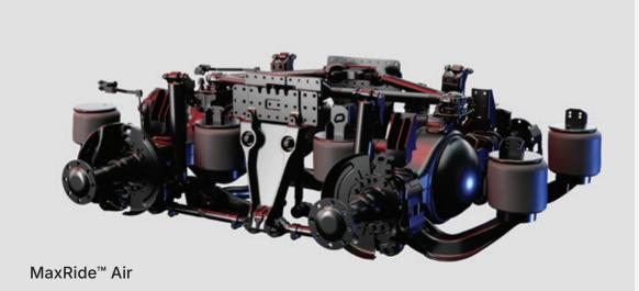
Advanced suspension utilizes electronically controlled rear suspension with eight tuned airbags to provide the most stable and best ride ever on a Mack Truck.
