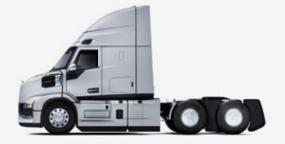
**44-Inch Mid-Roof Sleeper** 157" BBC. 13'6" overall height with roof fairing.
