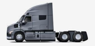
**64-Inch Mid-Roof Sleeper** 177" BBC. 13'6" overall height with roof fairing.
