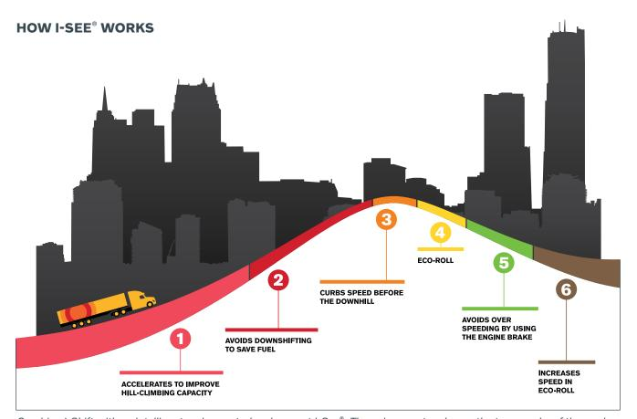
Combine I-Shift with an intelligent cruise control and you get I-See®. The unique system learns the topography of the road and manages shifting on known routes with hilly terrain to maximize fuel efficiency.
